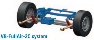
The VB-FullAir, a full-air rear-axle air-suspension, has an electronic system named VB-ASCU (VB-**A**ir **S**uspension **C**ontrol **U**nit), which automatically monitors and adjusts the height level of the vehicle. This constant monitoring and adjusting (independent of the load, in the longitudinal and lateral direction and relatively independent of centre gravity height) will automatically contribute to a safe vehicle behaviour and a better comfort. The vehicle may not been overloaded.
