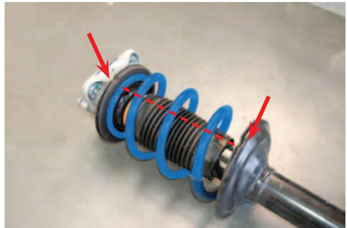
**EN** Place the VB-CoilSpring with the rubber coated end on the lower spring plate. Refit the top spring plate. Make sure the spring is placed correctly on the spring plates. The spring plates are marked. The notches should be in line.
