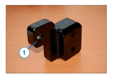
Secure the panhard ball-joint support to the *right* main spring. Put the bolts from the rear side to the front through the support as showed on the picture.
