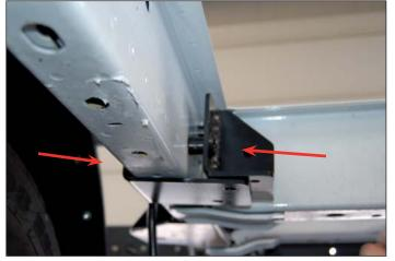
Secure these two parts to the chassis. Use Bolts, washers and nuts as showed in the picture.
