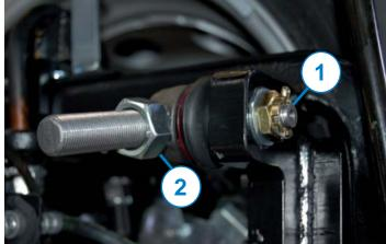
Next, fit the panhard rod to the ball-joint. Use antiseize compound to secure the rod to the ball-joint. However, do not tighten the nut (2) yet, as the length of the rod has to be determined later on.
