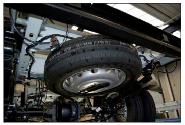
Next, remove the winch of the spare tire. To do so, remove the highlighted bolts. Only remove these bolts, later in this manual, the support is fitted back
