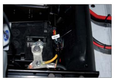
Disconnect the connector of the remote control in the seat console. Connect the calibrating unit (see picture) to the connector and put the fuses back in place.
