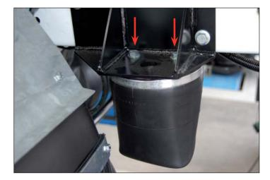
Pull the plug on the underside of the air spring down. Slide the piston over the plug of the air-spring at both sides of the vehicle. Secure it by screwing through the bottom of the mounting plate into the bottom of the air spring.
