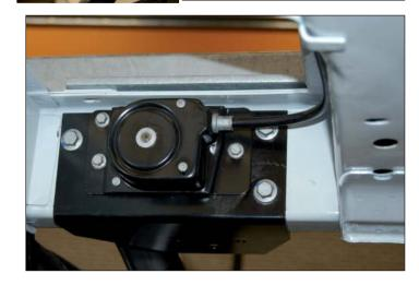
Next, fit the reaction-arm supports to the chassis. Also here counts, it might be necessary to remove some of the under-chassis protective wax.
