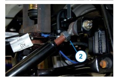
Measure the distance between the rim and the chassis (A) at both sides of the vehicle. These should be the same. If not, one can move the rear axle by changing the length of the panhard rod. Here counts: 1 turn equals 1,5 mm displacement.
