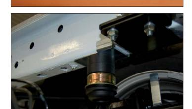
Next, fit both heightsensors in the supports. In the picture you can see the two heightsensor fitted. Pay attention to the difference between the left and right support. Fit the heightsensors with the plug pointing down and in opposite direction as the support.
