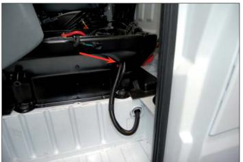
Start by connecting the fuse holders to the cable-tree. Slide the terminals of the red wires into a fuse-holder and put a 40 A fuse in it (Z1). Now slide the terminals of the yellow wires into the other fuse-holder and put a 7,5 A fuse in (Z2).
