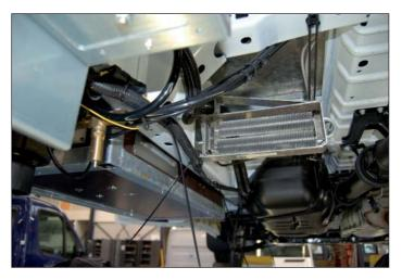
Lead the wiring harness through the same hole as the filling pipe of the fuel tank and lead it through the hole on the front side out of the beam (see inlay picture).
